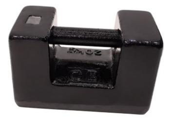
Cast-iron weights, conforming to OIML-R111 Recommendation in M1 class, suitable for legal metrology and industrial applications. The M1 accuracy class means these weights can be used for checking and calibrating scales and instruments in class III, up to 10.000e. Ideal for ISO quality weighing instrument verification.
