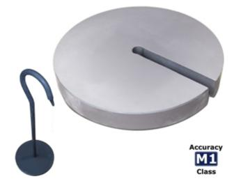
Disc weights suitable for legal metrology applications and the industrial sector and fully customisable. They have a groove and relief to allow them to interlock and keep them concentric; the slot allows them to be positioned on the bar. Their tolerances are those provided for OIML M1 class masses and therefore allow these weights to be used for the control and calibration of scales and class III instruments up to 10.000e.
